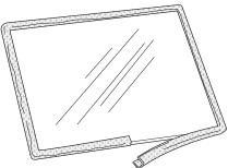
Figure 41. Wrap the gasket around the glass panel.
