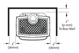
Figure 3. Parallel Installation Clearances.
