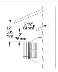
Figure 21. Termination Clearance to overhangs.
