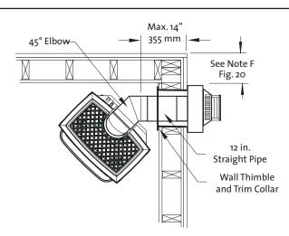
Figure 19. Corner Installation with 14" Snorkel Termination.
