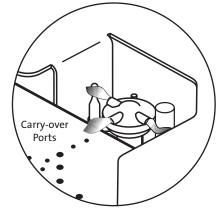
*Figure 37a. Proper pilot flame appearance relative to burner carry-over porting.*
