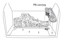
Figure 33. Install Right Log
