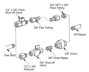
Figure 28. Supply valve connection fittings.
