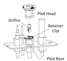
Figure 26. Pilot orifice removal and replacement.
