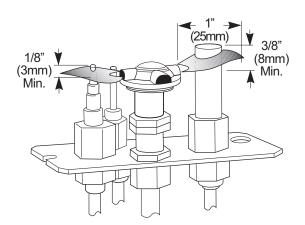
Figure 37. Proper pilot flame appearance.
