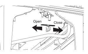
Figure 22. Locate and remove the Air Shutter wingnut from under the right side of the stove.
