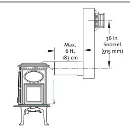
Figure 18. Maximum Horizontal with 36" Snorkel Termination.
