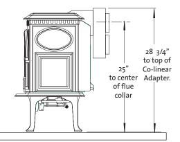
Figure 15. Simpson Dura-Vent #923GCL Co-linear Adaptor. Subtract 2 1/4" for Short Legs.
