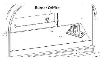
Figure 24. Change the Burner Orifice.
