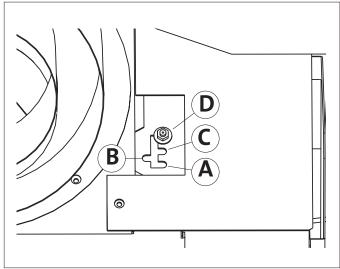
*Figure 6. Exhaust restrictor positions - viewed from front with top plate removed.*
