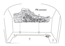
Figure 32. Engage the holes in the underside ot the Rear Log with the two pegs in the burner skirt.
