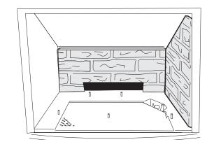
Figure 50. Install Side Panel
