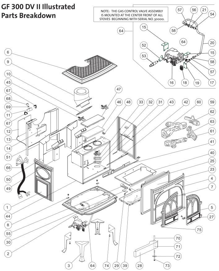
Figure 52. Illustrated Parts Breakdown - GF 300 DV II Allagash
