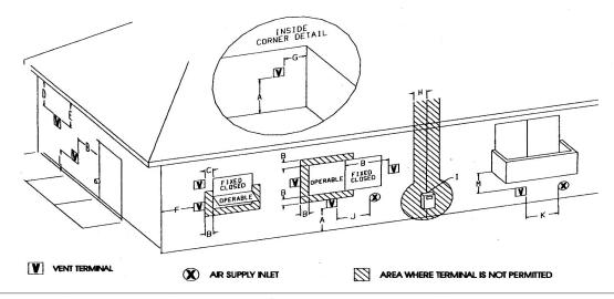
Figure 20. Vent Terminal Clearances - ANSI Z21.88-2002, CSA 2.33-2002, and National Fuel Gas Code.
