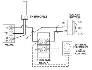
Figure 31. Accessory wiring diagram.
