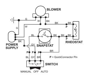
Figure 46. Blower Wiring Diagram
