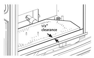
Figure 25. Correct Burner Position.
