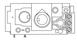
Figure 29. Pressure test points.
