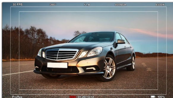
SDI Overlays set to display on a monitor attached to the SDI output
