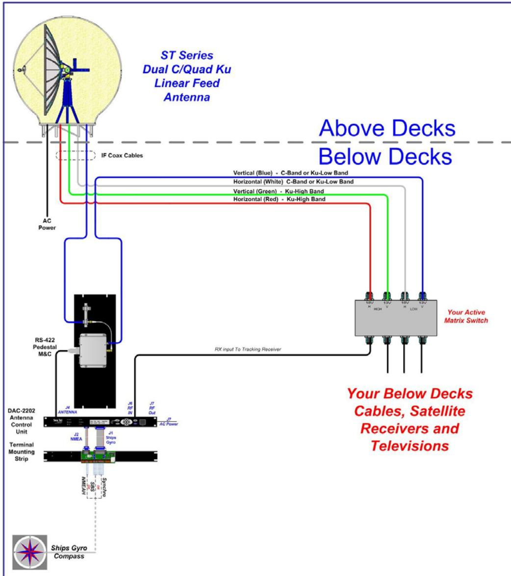
Figure 1-1 TVRO Simplified Block Diagram
