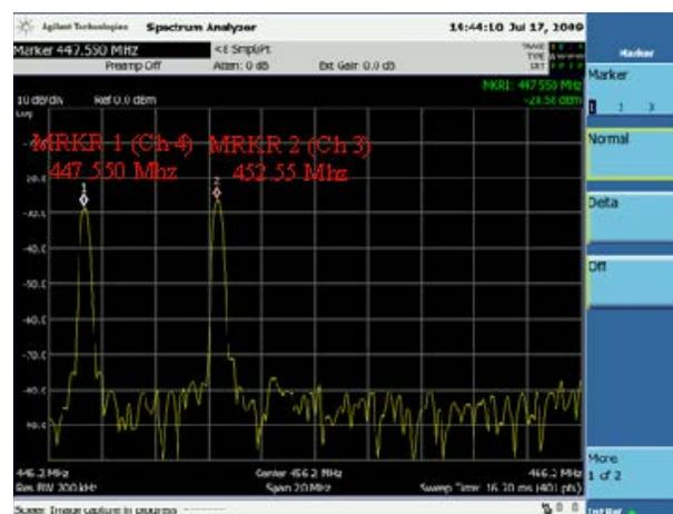
Figure 8 BDE Modem Transmit Frequency Markers
