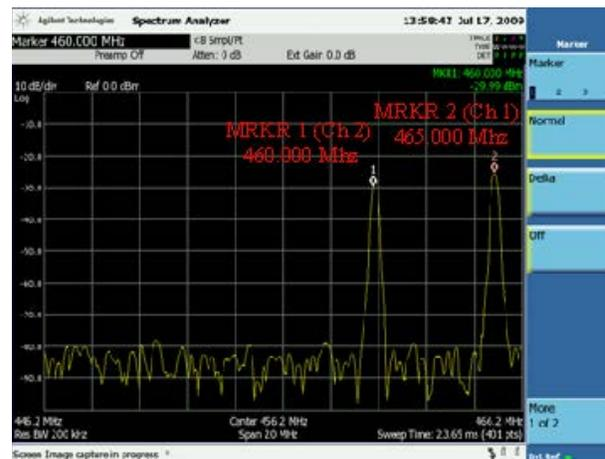
Figure 7 ADE Modem Transmit Frequency Markers
