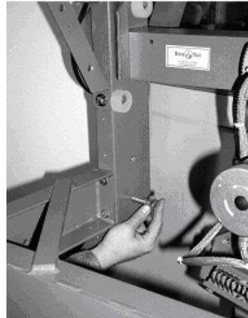
3. Hook one end hook of the nylon strap to bolt in elevation beam as shown in Figure 2.
