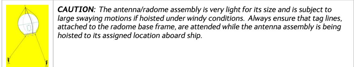
1. Assure that the antenna is restrained before hoisting. Check that all nuts on the base frame assembly are tightened according the torque values listed below:
