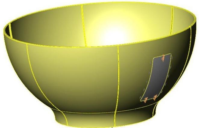
23. Attach four radome lifting brackets (PN 122848), or other lifting arrangement, evenly spaced around the bottom of the lower panel assembly.
