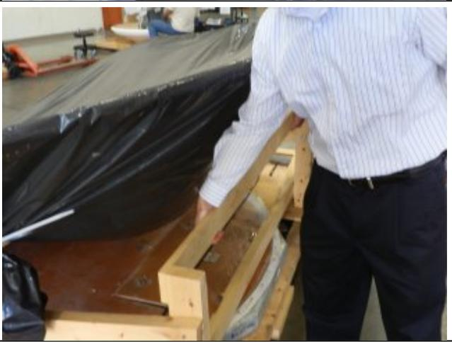
4. Allow the drop down legs on the reflector support to swing down to support the structure in the raised position.
