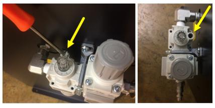
3) Fill FRL using Snap-On AirOil #IM6 or equivalent. Oil to be filled to the MAX line marked on reservoir. If unit does not have MAX line mark, reservoir should be 80% full.
