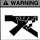
Keep clear of pinch points when lift is moving.
