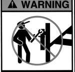
Do not overide self-closing lift controls.
