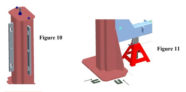
**AWARNING** IF THE TOWERS ARE LEANING INTO THE LIFT, THE CROSS MEMBERS CAN BECOME WEDGED INTO THE TOWERS AS THE LIFT RAISES.
