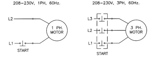
Figure 65 – Electrical Diagram
