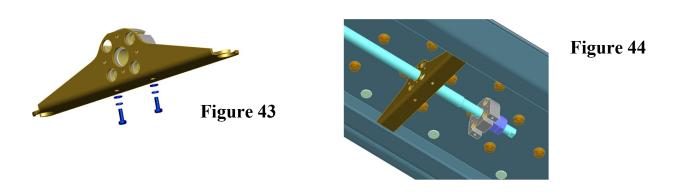
**NOTE:** THE CYLINDER ROD MUST BE FULLY EXTENDED IN ORDER TO ATTACH THE NON-THREADED ENDS (SLEEVES) OF THE CABLES TO THE CABLE FLANGE ON CYLINDER ROD. USE COMPRESSED AIR IN THE SHOP AND AN AIR NOZZLE AT THE BREATHER END TO EXTEND THE CYLINDER ROD. USE CAUTION AND PROTECTIVE EQUIPMENT WHEN WORKING WITH COMPRESSED AIR.
