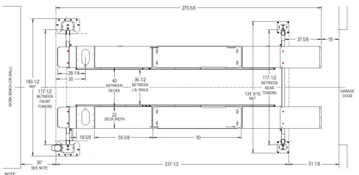
If using this lift in conjunction with an alignment system, consult aligner manual for manufacturer's minimum recommended distance to front turn table, and adjust this dimension accordingly.
