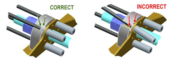
Figure 46.a, b. Seating the cable in the cable flange slots
