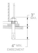
**NOTE:** The 3/4"  $\times$  7" lg. wedge anchor bolts supplied must have a minimum embedment of 4" into the concrete floor.
