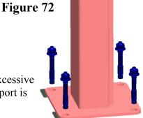
• Torque all anchor bolts to 55 ft-lbs. (75 Nm), continually checking that the column is level as you proceed. **Do not exceed tightening torque.**
