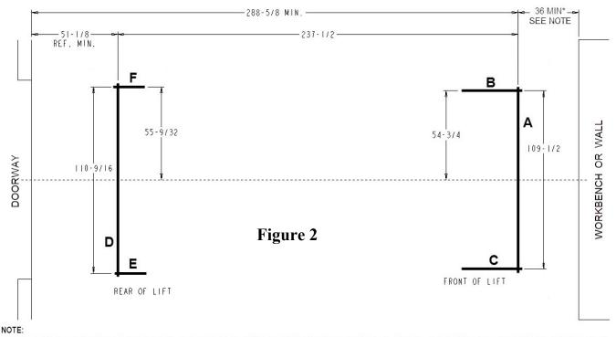
If using this lift in conjunction with an alignment system, consult aligner manual for manufacturer's minimum recommended distance to front turn table, and adjust this dimension accordingly.
