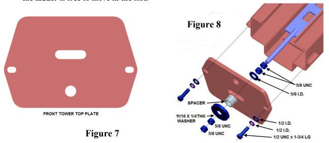
• Stand up tower, move into position at the front of the lift (see Fig.10), and line up with lines "A" and "B". **Handle tower and front cross-member only by the tower**. As the cross-member is only restrained to the tower by safety locks, care must be taken when handling tower with cross-member.
