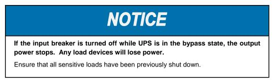
To completely stop the UPS, open/turn off the main input breaker MCCB, the secondary Input breaker if available, and the external battery cabinet breaker (if available).
