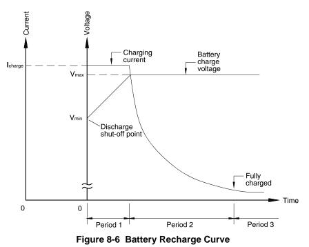
The recharge process consists of three steps.
