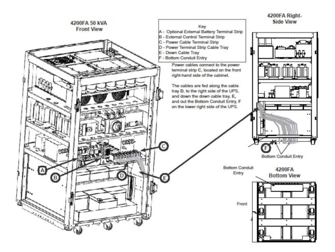
Note: Cabinet show with batteries, cabling is the same for units with internal batteries, internal transformers, and neither internal batteries nor transformers.
