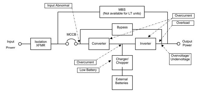
Figure 11-1 UPS Electrical Protection Sense Points
