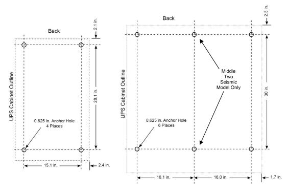
Figure 4-4 Anchoring Pattern for Basic and Seismic 50kVA (C-Channel Feet) See Appendix A for fastener details.
