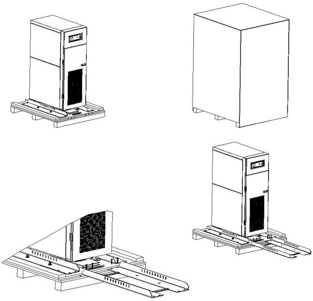
4. Save the loading rails for seismic anchoring of the UPS. See pg. 14.
