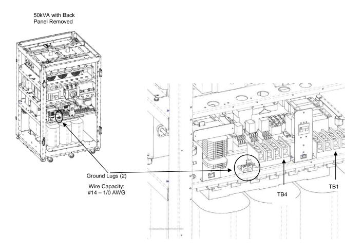
Figure 6-6 Terminal Board Locations – 50KVA
