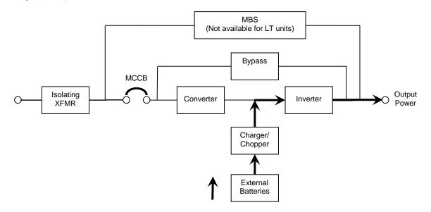
Figure 8-4 Power flow in battery backup mode
