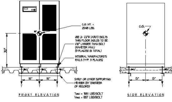
LOADS: PER 2010 CALFORNIA BUILDING CODE SECTION 1613A AND ASCE 7-05 SECTIONS 12 AND 13. (STRENGTH DESIGN IS USED) (SDS = 200, 8.p = 25, 1p = 15, Rp = 6.0) WEIGHT = 2648 LBS
