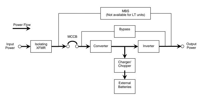
Figure 8-1 Power flow in AC Input Mode
