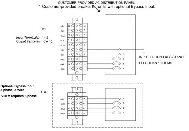
Figure 6-1 Power Cabling for 15-30kVA Units with Internal Batteries
