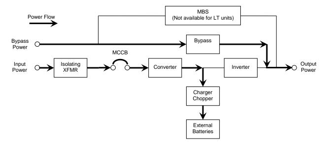
Figure 8-3 Power flow in Bypass mode for the Alternate Input Models
