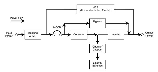
Figure 8-2 Power Flow in Bypass Mode
