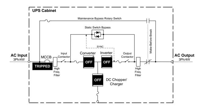
Figure 9-2 Effect of EPO Activation
