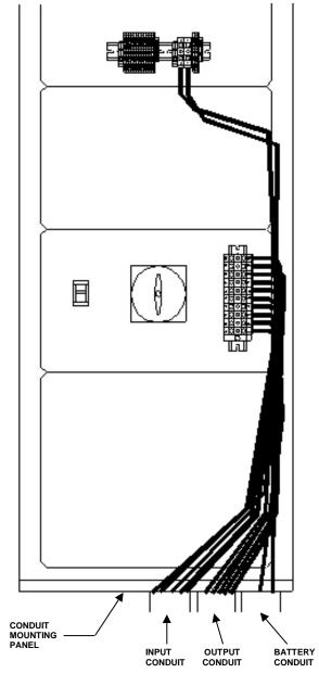
Figure 6-3 15030kVA Cable Routing
