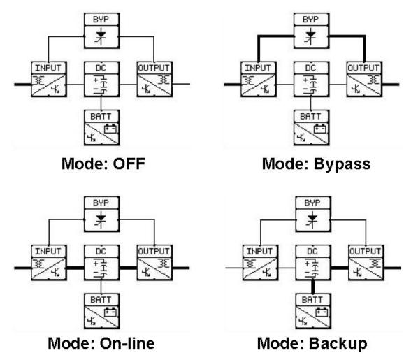
Figure 9-13 Mimic Display Current Flow Indicator
