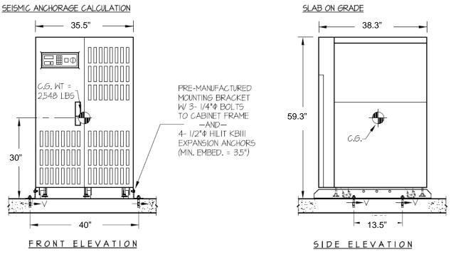
Figure 4-3 Anchoring for 50kVA with Casters
