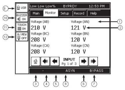
Figure 9-7 Monitor Display Layout
