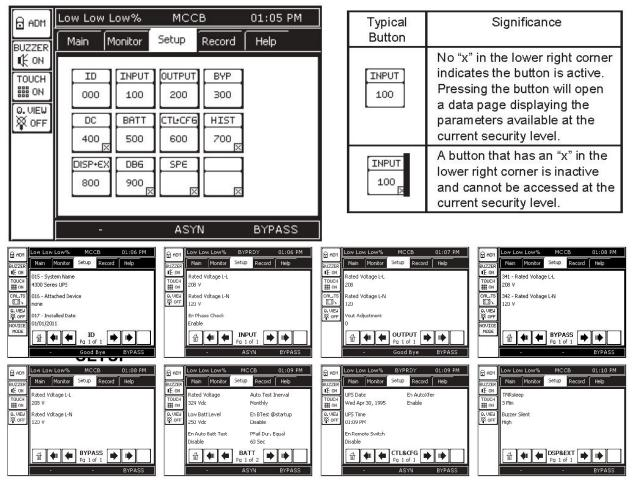
Figure 9-14 Setup Tab
