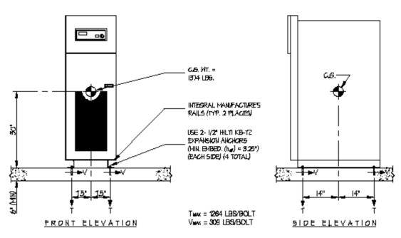
LOADS, PER 2010 CALFORNIA BUILDING CODE SECTION 1613A AND ASCE 7-05 SECTIONS 12 AND 13. (STRENGTH DESIGN IS USED) (SDS = 200, 8p = 25, 1p = 15, Rp = 60)
