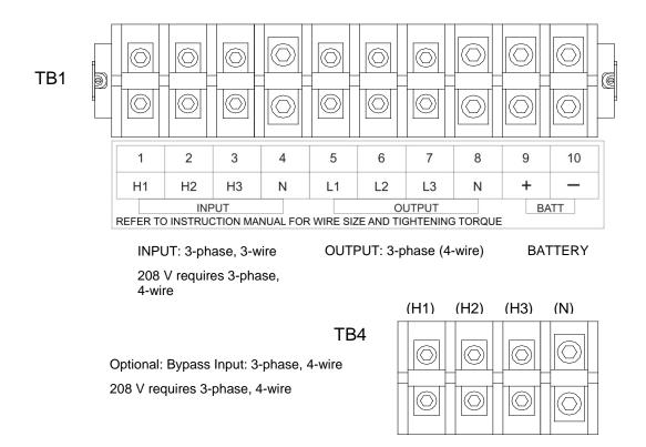
Figure 6-5 Power Terminals - 50kVA
