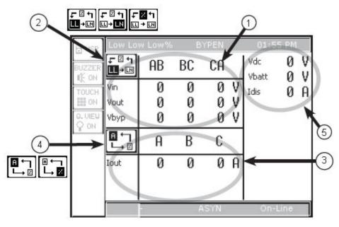
Figure 9-10 Quick View Display Layout
