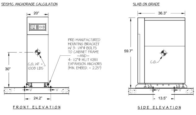
Figure 4-2 Anchoring for 15-30kVA with Casters
