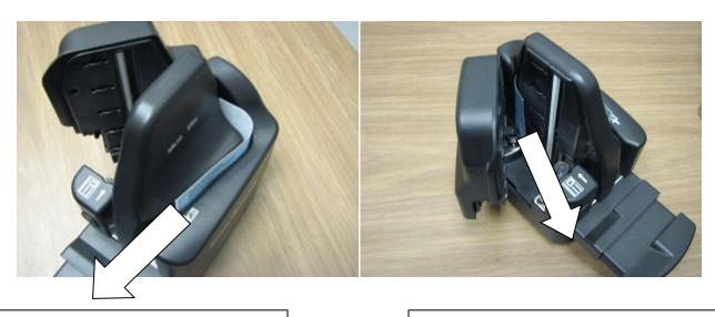
Pull out stopped document from the frontparallel to the track Pull out stopped document-open Image cover & pull out parallel to the track
