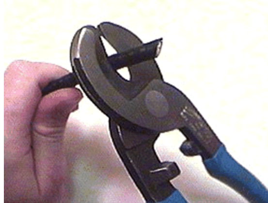
Figure 8. Coax Cable Cutting Technique
