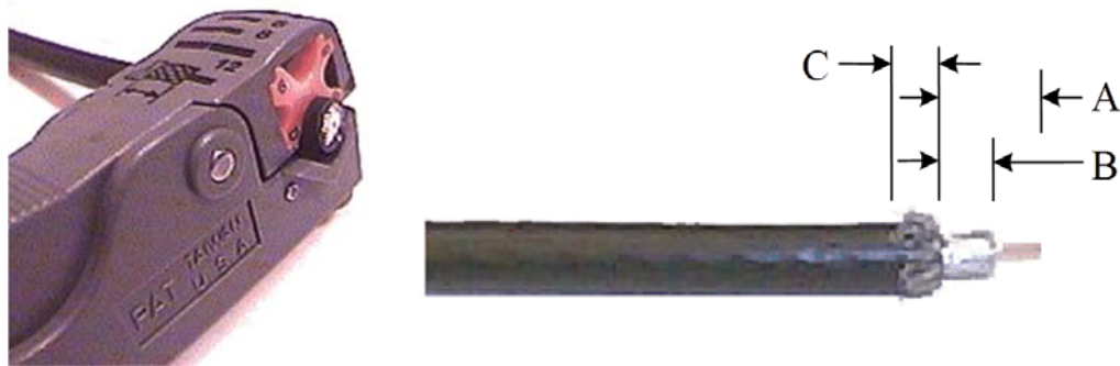
Figure 9. Cutting Technique for Removing Foil in the Braid
