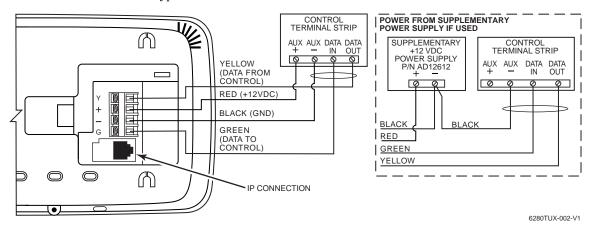
**IMPORTANT:** When the keypad is powered from an auxiliary power supply, always apply power to the control panel <u>first</u> and then the keypad. Failure to observe this sequence results in improper operation of the keypad and may result in an ECP Error indication.
