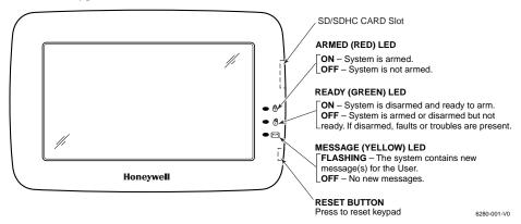
**NOTE:** If the Screen Blackout feature (\*EN50131 Display) is enabled (see below) the keypad returns to the "Home" screen and the "Armed" and "Ready" status LEDs turn OFF after 30 seconds. The keypad will remain in this state until a valid user code is entered.
