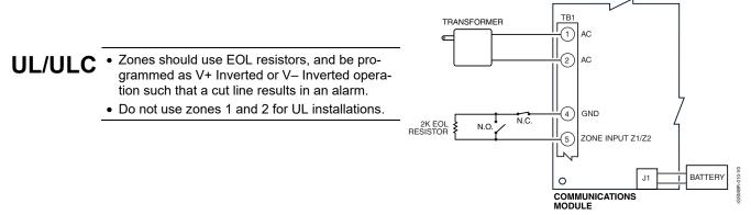
Wiring the Zone 1 Input for EOL Supervised N.O./N.C. Triggers
