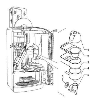
3. Gently push downward on section 4 and firmly pull out the centre section 3 to remove. Clean 2, 3 and 4 of all parts of powder residue using warm water and detergent. Section 5 may be cleaned by rotating then pulling outward to remove. Reassemble in reverse order. **Do not** clean any parts in a dish washer as this will cause damage.
