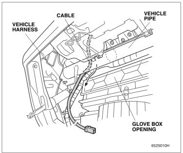
41. Route the cable along the vehicle harness to the right side, and secure it to the vehicle harness with four wire ties.
