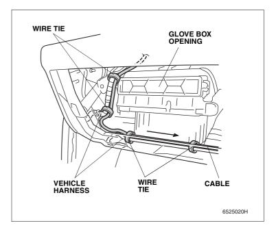
42. Route the cable to the audio opening from the glove box opening as shown. Align the cable connector with the vehicle 17-pin connector, and bundle up the excess cable and secure them to the vehicle harness with the wire ties.
