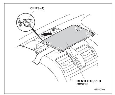
11. Remove the center cover (five clips and disconnect a vehicle connector).
