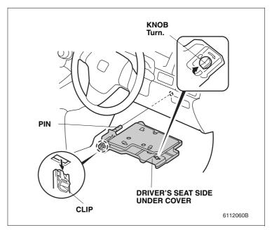
14. Remove the driver's seat side lower cover (seven clips).
