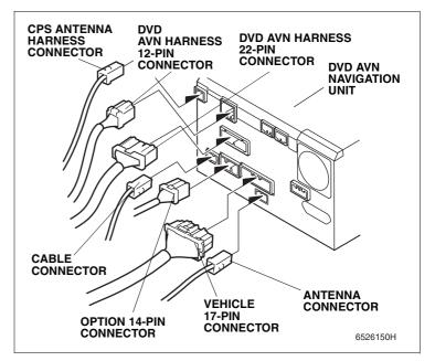
68. Install the DVD AVN navigation unit with four screws removed in step 12.
