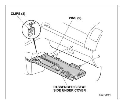
6. Remove the glove box (dumper and two screws).
