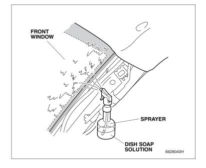
24. Fold up one side of the backing of the film antenna, then spray the dish soap solution to the adhesive surface of the film antenna.
