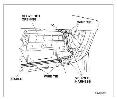
42. Route the cable to the audio opening from the glove box opening as shown. Align the cable connector with the vehicle 17-pin connector, and bundle up the excess cable and secure them to the vehicle harness with the two wire ties.
