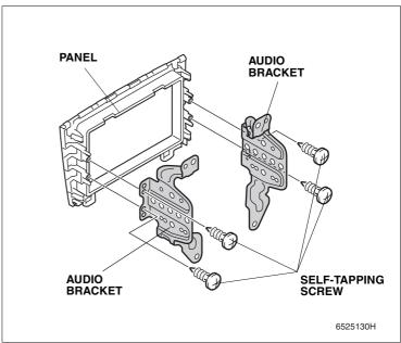
66. Insert DVD AVN navigation unit into the panel, and install it to the audio brackets with eight screws removed in step 64.
