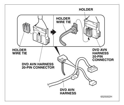
52. Plug the DVD AVN harness 20-pin connector to the vehicle 20-pin connector.
