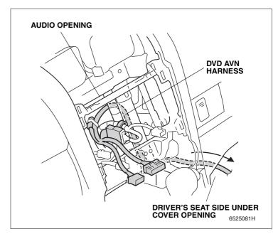
55. Route the DVD AVN harness along the vehicle harness to the right side, and secure it to the vehicle harness with a wire tie.
