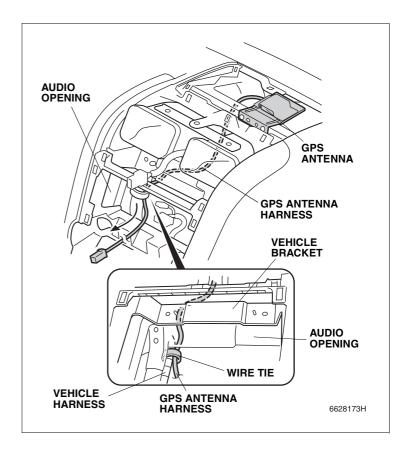
49. Align the GPS antenna harness connector with cable connector, bundle up the excess GPS antenna harness, and secure them to the vehicle harness with a wire tie.
