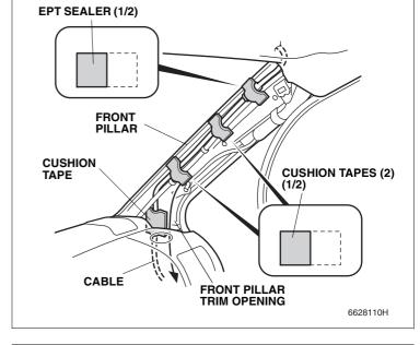
40. Pull out the cable at the glove box opening, and route the cable along the vehicle harness as shown.
