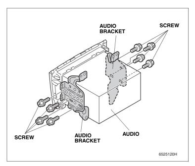
65. Install the audio brackets removed in step 64 to the panel with the four self-tapping screws.
