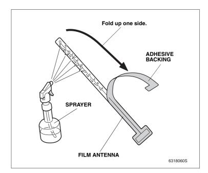
25. Attach the film antenna to the inside of the front window. Align the film antenna with end line of the black ceramic paint as shown, and Align the end line of the film antenna with the end line of the black ceramic paint at a distance of 5 mm.
