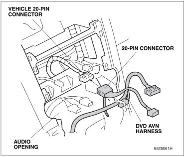
53. Install the holder wire tie to the vehicle harness in the audio opening as shown.
