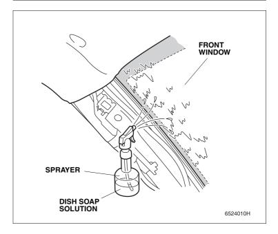
24. Fold up one side of the backing of the film antenna, then spray the dish soap solution to the adhesive surface of the film antenna.
