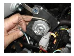
4. Disable Exhaust Valve Servo Motor
