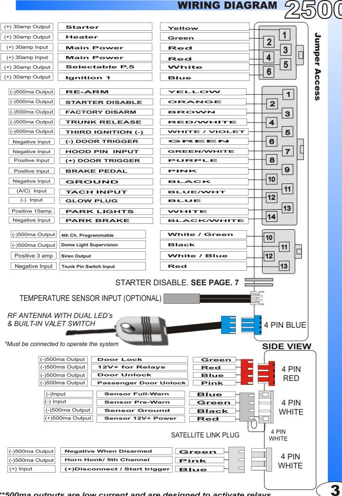
\*\*\*500ma outputs are low current and are designed to activate relays
