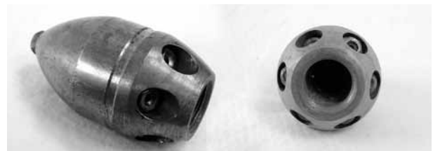
Figure 9-6 Nozzle with jet holes around the circumference, 2.5 kg
