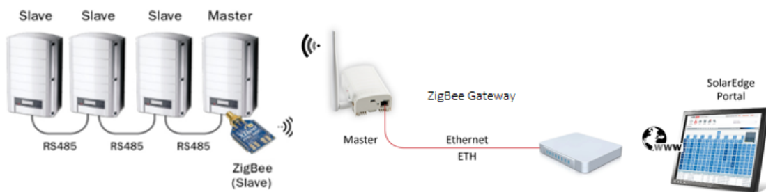
Figure 13: Multiple devices, RS485 bus , ZigBee server connection
