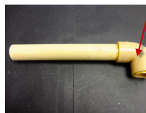
Image 5 & 6. Thermal expansion / contraction damage to fitting
