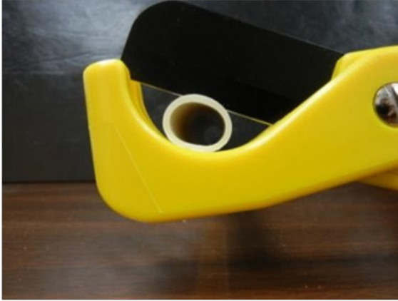
Image 19. Scissor Cutter: not recommended for CPVC
