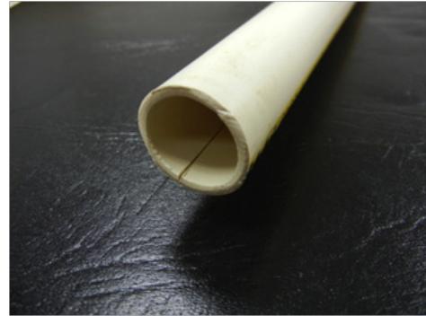
Image 17. Damaged Tubing End
