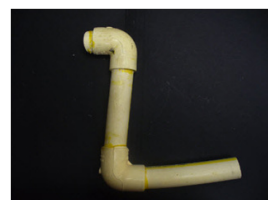
Image 7. Pipe under excessive flexural stress
