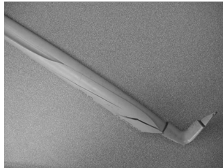
Image 25. Examples of damage resulting from freezing
