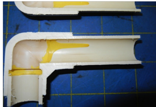
Image 18. End crack shown in cutaway
