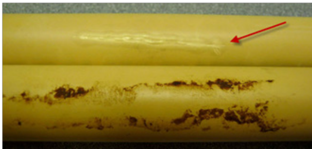
Image 2. Damage from plasticizer contact
