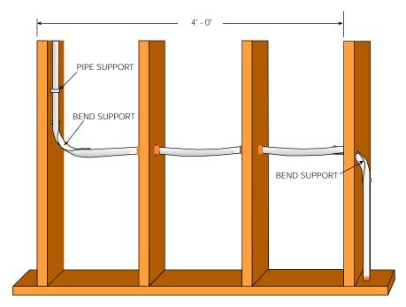
Allow  $\frac{1}{6}$ " to  $\frac{3}{16}$ " of slack per foot of hePEX pipe. (4' x  $\frac{3}{16}$ " =  $\frac{3}{4}$  " of slack.)
