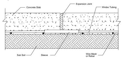
1. If the tubing must remain in the slab, wrap the tubing with a pipe sleeve or a larger diameter tubing for 6" on both sides of the expansion joint.
