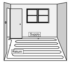
**Single Wall Serpentine** — Use when a single wall represents the major heat loss of the zone. The supply is fed directly to the high heat loss wall and then serpentined toward the lower heat loss area. Start tubing runs 6" from walls or nailing surfaces. A 6" on center tubing run is often installed along outside walls to improve response time.
