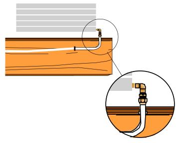
Wirsbo hePEX<sup>™</sup> plus should not be placed in direct contact with copper pipe or copper fittings. Use Wirsbo transition fittings to connect Wirsbo hePEX<sup>™</sup> plus to copper pipe, copper fittings, or to dry seal (NPT) pipe threads.
