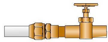
Use conversion nipples to connect Wirsbo hePEX™plus to NPT pipe or fittings
