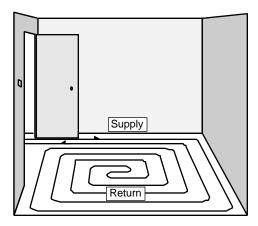
**Counter Flow** — Use when the heat loss for the room is evenly distributed throughout the entire room or the major heat loss is to the floor. The supply is fed along the exterior of the room spiraling inward with the return paralleling it from the center of the room. Start tubing runs 6" from walls or nailing surfaces. A 6" on center tubing run is often installed along outside walls to improve response time.
