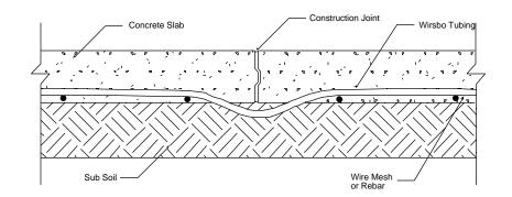
1. Dip tubing under joint below the slab.
