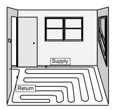
**Double Wall Serpentine** — Use when there are two adjacent walls representing the major heat loss of the room. The supply is fed directly to either of the heat loss walls and then serpentined toward the lower heat loss area in an alternating pattern against the two heat loss walls. Start tubing runs 6" from walls or nailing surfaces. A 6" on center tubing run is often installed along outside walls to improve response time.
