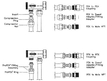
**NOTE:** The <sup>3</sup>/<sub>4</sub>" connection will accommodate any QS20 style compression nut used for <sup>3</sup>/<sub>8</sub>", <sup>1</sup>/<sub>2</sub>" and <sup>5</sup>/<sub>8</sub>" Wirsbo PEX tubing. The QS20 compression nut used for <sup>3</sup>/<sub>4</sub>" PEX tubing will not connect directly onto the <sup>3</sup>/<sub>4</sub>" outlet.
