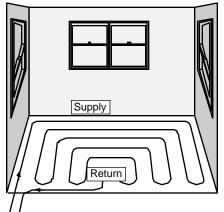
**Triple Wall Serpentine** — Use when there are three walls representing the major heat loss of the room. The supply is fed along the heat loss walls in an alternating pattern and serpentined toward the lower heat loss area of the room. Start tubing runs 6" from walls or nailing surfaces. A 6" on center tubing run is often installed along outside walls to improve response time.
