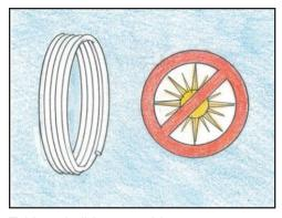
Tubing shall be stored in a way to protect the system from mechanical damage (slitting, puncturing, etc.). Tubing and fittings shall be stored undercover for cleanliness and to avoid exposure to sunlight. Consult manufacturer for recommended limits for outside storage.
