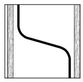
Expansion loops (left) and offsets (right) also provide means to accommodate tubing expansion and contraction. Refer to the PEX tubing manufacturer's installation instructions for more detailed information on expansion compensation techniques.
