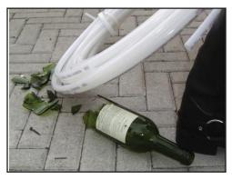
Do not drag the tubing over rough terrain, rocks, or any surface that can cut, puncture, or damage the tubing wall.
