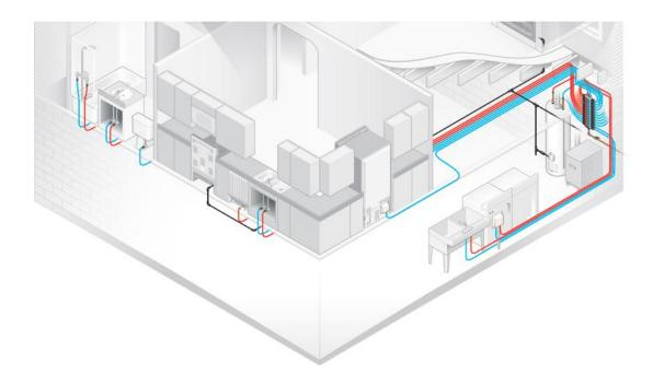
This drawing represents a typical manifold system
