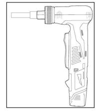
**IMPORTANT**: Rotation of the expander head in either direction after every expansion is necessary to provide smooth and even expansion of the tubing. If you fail to reposition the head after each expansion, the segments of the tool head may cause deep grooves in the tubing, which could result in potential leak paths.
