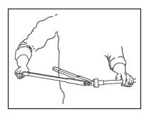
4. When using the hand expander tool, place the free handle of the tool against your hip, or place one hand on each handle when necessary. Fully separate the tool handles and insert the expander head into the end of the tubing until it stops. Be sure you have the correct size expander head on the tool. Full expansion is necessary to make a proper connection. Bring the handles together to expand. Separate
