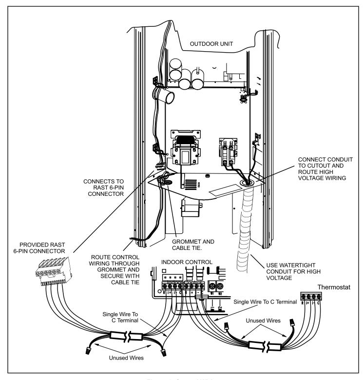
Figure 6. Control Wiring
