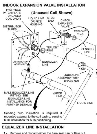
3 - Install one of the provided Teflon® rings around the stubbed end of the check expansion valve and lightly lubricate the connector threads and expose surface of the Teflon® ring with refrigerant oil.
