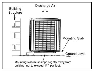
Figure 1. Slab Mounting
