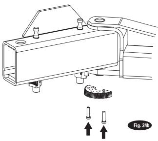
**NOTE**: Once arm is installed in yoke, pull up actuator pin and swing arm fully around, being sure that the Restraint Gear and Gear Block always stay aligned. If they do not stay aligned, remove restraint gear and install in the opposite position.
