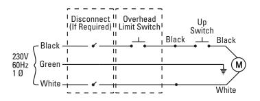
Note: 60Hz. Single phase motor CAN NOT be run on 50Hz. line without a physical change in the motor.
