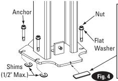
NOTE: Use rectangular shims at inside edge of baseplate. Use constructions adhesive or silicon cement to hold shim in place. INSURE shims are held tightly between base plate and floor after torquing anchors.
