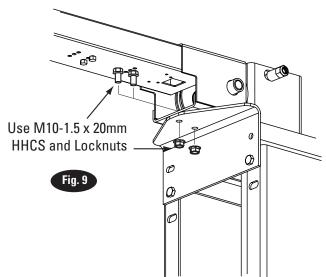
10. Power Unit: First install a star washer onto all of the (4) 5/16"-18NC x 1-1/2" HHCS. This is very important for grounding. Put the (4) 5/16"-18NC x 1-1/2" HHCS thru holes in power unit bracket, Fig. 9. Mount unit with motor up to column bracket and install (4) 5/16" star washers and 5/16" Nuts. Install and hand tighten fitting to pump until 0-ring is seated. Continue to tighten the locknut until the nut and washer bottom out against the pump manifold.
