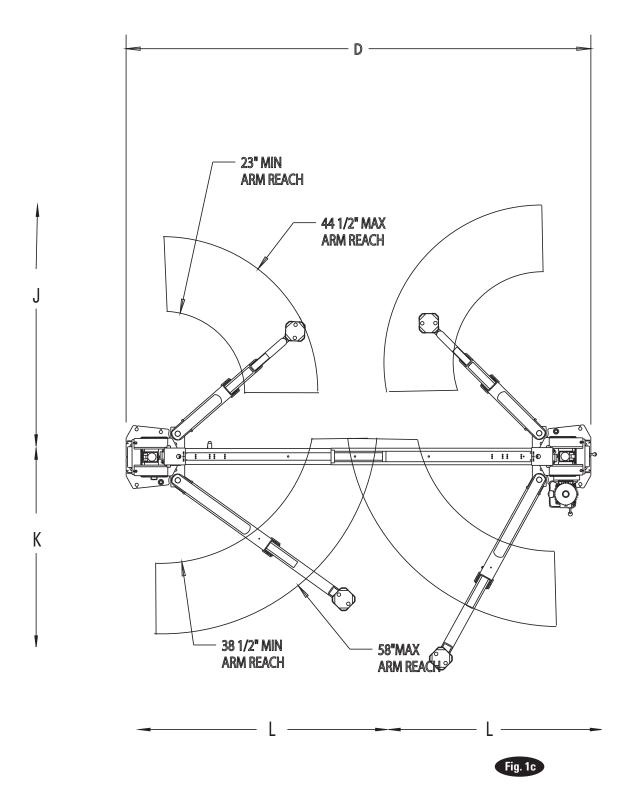
1. Lift Location: Use architects plan when available to locate lift. Fig. 1a & Fig. 1b shows dimensions of a typical bay layout.
