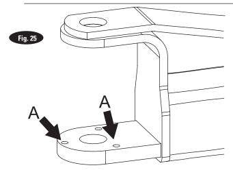
Use holes marked "A" for Left Front and Right Rear.
