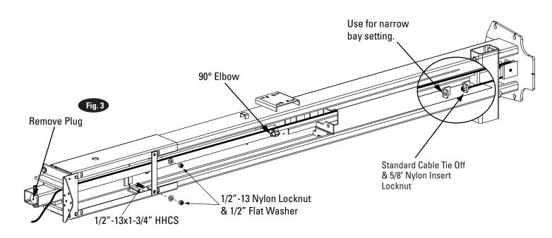
6. Lift Setting: Position columns in bay using dimensions shown in Fig. 1a & Fig. 1b. Place column with power unit mounting bracket on vehicle passenger side of lift. Both column base plate backs must be square on center line of lift. Notches are cut into each base plate to indicate center line of lift. Use appropriate equipment to raise carriage to first latch position. Be sure locking latch is securely engaged.
