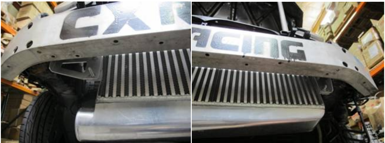
Left and right Intercooler mounting bracket:
