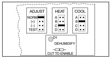
Figure 2. Motor Board Taps and Dehumidify Resistor
