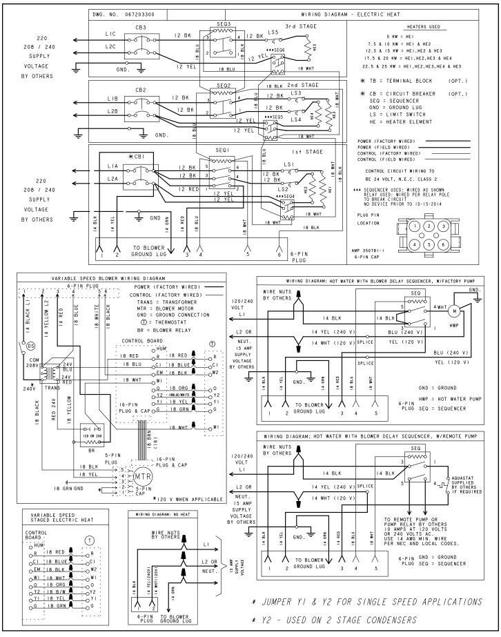
Figure 4. Wiring Diagram Variable Speed Blower
