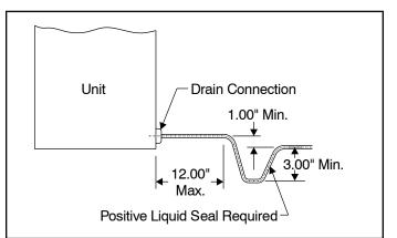
Figure 1. Typical Condensate Drain Connection
