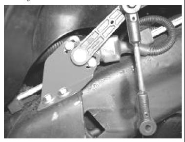
67. Install the FT20098 brake line extension tab using the original bolt and the supplied 5/16" hardware. SEE PHOTO IN NEXT COLUMN.
