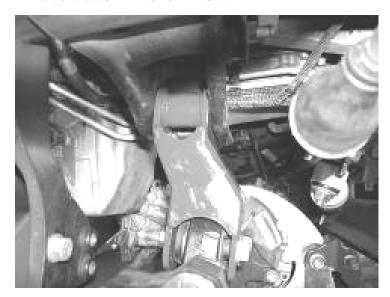
24. Place the differential housing into the Fabtech rear crossmember using the supplied ½" x 4 ½" bolt, nut, and washers along with the supplied large FT55-1 washers attach the differential. SEE PHOTO ON NEXT PAGE.
