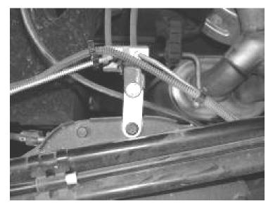
68. Raise the floor jack supporting the rear axle and slide the lower mount of the track bar into the new bracket on the axle. Torque to 105ft. lbs. SEE DIAGRAM BELOW.
