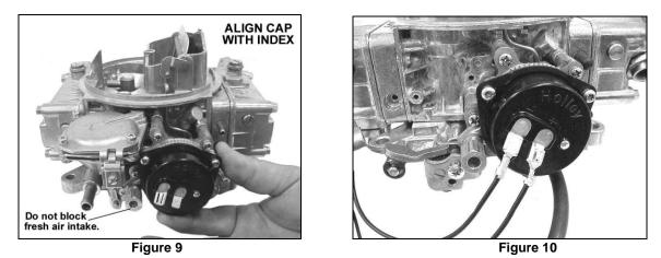
NOTE: Do not block the fresh air intake, as shown by the arrow in the photo above.
