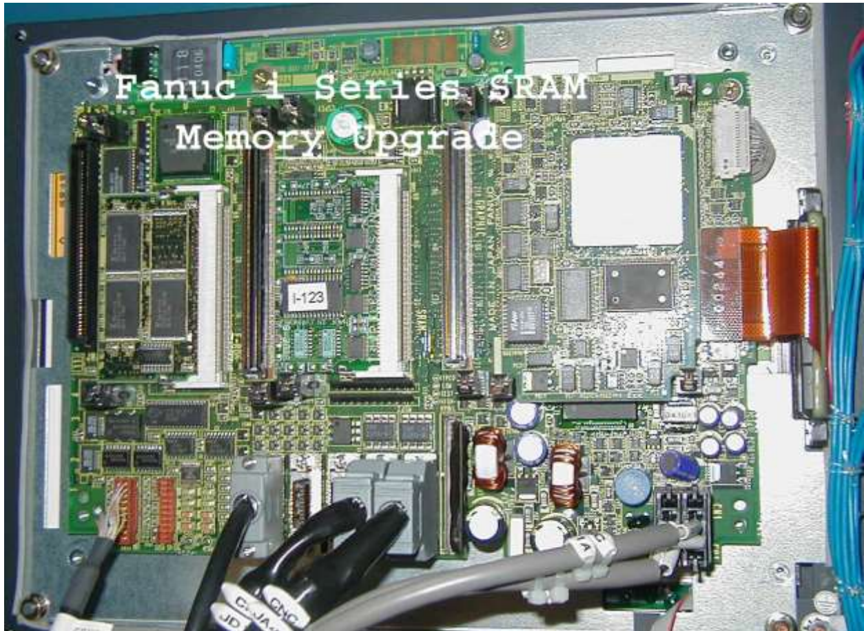
After removing the yellow case and the left 2 covering cards, you will see the SRAM module (DIMM) in the center.
