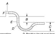
A. Drain connection B. 2" (5.1 cm) minimum C. 3" (7.6 cm) minimum D. Positive liquid seal (required) E. Flexible tubing, hose or pipe F. Unit
