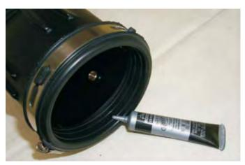
95. Push the bellows end of the air tube assembly on to the air box first, and then install the remaining end with the coupler on to the throttle body. Tighten all clamp screws securely.
