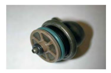
56. Using a small amount of grease or oil lubricate the two O-rings on the fuel pressure regulator and push it into the new supplied fuel manifold as shown.
