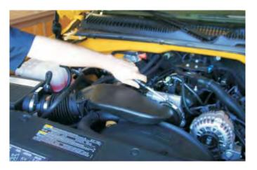
10. Remove the duct assembly by lifting it out. Sight shield and duct assembly will not be reused.
