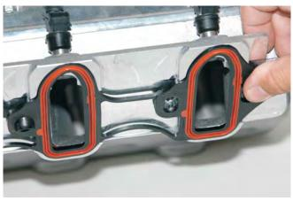
49. Remove the stock MAP sensor from the stock intake manifold by pulling back on the two tabs and lifting the sensor out. Ensure that the orange MAP sensor seal is not damaged, as it will be used.
