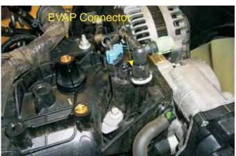
25. Lift the electrical harness from the top of the engine and set off to the side.
