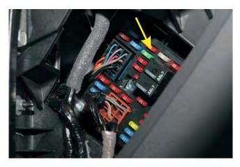
113. Remove the cover from the "Exterior Fuse Panel" located under the hood on the drivers (left) side. Remove the six fuses labeled SEO B1, SEO IGN, INFO, SEO B2, RADIO and RADIO AMP. Download the Micro Tuner following the instructions that came with the Micro Tuner.
