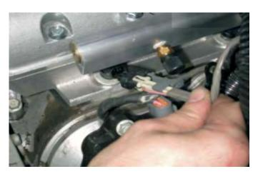
80. Attach one end of the ¼" coolant hose supplied to the new steam vent pipe and the other end to the barb on the bottom of the throttle body with the clamps supplied. Attach the original steam vent hose and clamp from the radiator to the remaining barb on the bottom of the throttle body. Refill the cooling system with either the coolant you removed in step 6 or with fresh coolant. Securely tighten the reservoir cap.
