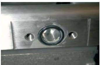
59. Install the assembled fuel manifold to the driver side fuel rail using the two new supplied 6mm bolts. Using a 10mm socket wrench torque the bolts to 106 lb-in. (Be careful not to pinch the O-ring.)
