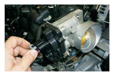
22. At the rear of the of the intake manifold disconnect the Manifold Absolute Pressure (MAP) sensor connector by gently raising the gray plastic retaining clip and then pull free the connector itself.
