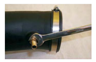
94. Using some of the O-ring grease supplied, apply a light coating of grease on the inside of the coupler.
