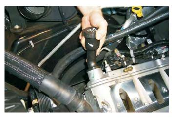
42. Install the short oil filler neck supplied by inserting it into the valve cover and rotating it 180 degrees clock-wise. Transfer the oil fill cap from the long neck to the new short one.
