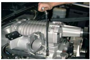
75. Push the fuel line connector on to the fuel manifold. Ensure that the fuel line is pushed all the way on. Pull on the connector to check that it is secure, you should not be able to remove the connector unless you use the removal tool.
