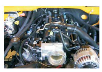
20. Disconnect the eight fuel injector connections by gently pulling up on the gray plastic release trigger on the connector and then pulling firmly on the connector itself.
