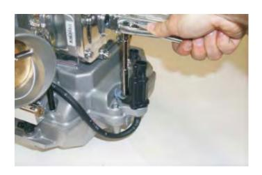
66. Remove the one bolt directly below the alternator and factory GM idler with a 15mm socket wrench.
