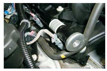
21. Disconnect Electrical Throttle Control (ETC) connector from the throttle body by removing the gray plastic locking tab first, then squeeze and pull free the ETC connector itself.
