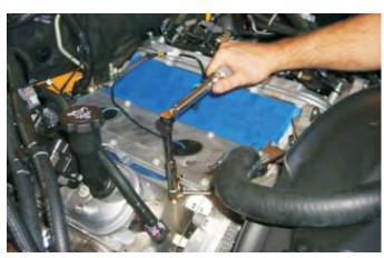
47. Using the new supplied 16" x 3/8" PCV vacuum hose, connect one end to the PCV valve as shown and lay the other end of the hose off to the driver side, out of the way. (To be connected in a later step.)
