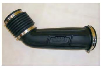
93. Install the brass barb into the threaded port in the bottom of the air tube with a 14mm wrench. Do not over tighten!
