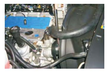
38. Using a 15mm socket wrench remove the three bolts holding the factory belt tensioner to the bracket and remove the tensioner.
