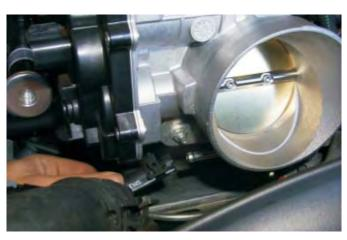
16. Remove the PCV vent hose from the throttle body or intake manifold on passenger side. (Depending on year.)
