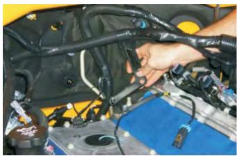
35. Using a 10mm socket wrench remove the two coolant vent pipe bolts.
