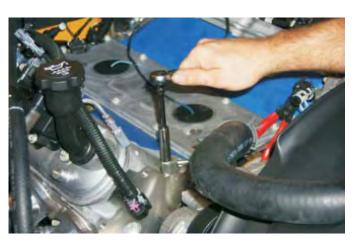
36. Remove the vent pipe assembly. (Make sure that the O-ring gaskets did not stick to the cylinder heads, if so remove them.)
