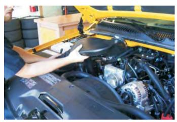
11. Unplug the electrical connector to the MAF sensor.
