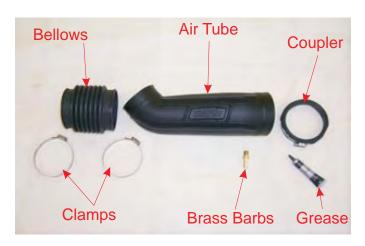
92. Assemble the bellows and coupler to the air tube. Note: The position of the clamp screws. The screws must be facing up so that you can install the assembly on the vehicle.
