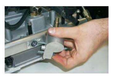
60. Using the small 3/16" hose supplied, connect one end to the small barb on the pressure regulator. Connect the remaining end of the hose to the barb at the left rear of the supercharger manifold.
