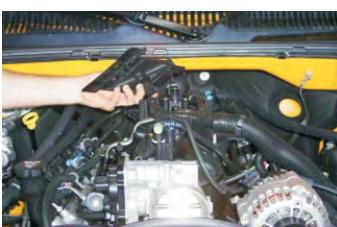
19. Disconnect the following electrical and hose connections from the intake manifold area.
