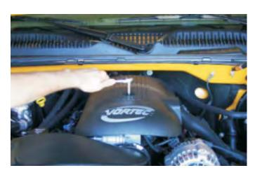
8. Lift plastic shield from top of engine.
