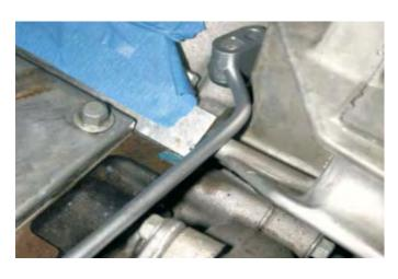
44. Use a felt tip marker and mark the alternator bracket were the coolant vent pipe hits as shown.
