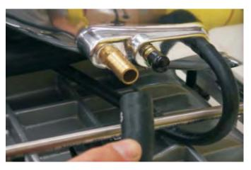
54. Remove the stock fuel pressure regulator from the fuel rail by disconnecting the vacuum hose, pulling off the spring clip and pulling the regulator out. Be careful not to lose any of the small O-rings on the regulator.
