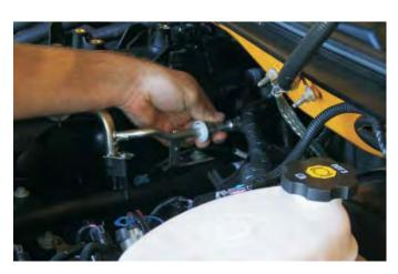
28. Disconnect the EVAP vent tube from the solenoid by squeezing the retainer, then release the tube from the solenoid. Follow the same procedure on the other end of the EVAP vent tube and remove the tube from the vehicle.
