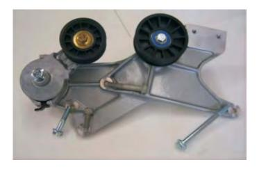
68. In the original tensioner location, install the new tensioner support bracket. Torque all mounting fasteners to 40 lb-ft.
