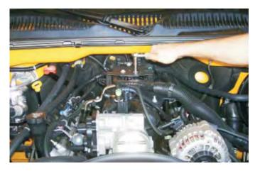
18. Open the large electrical harness retainer clip, then using a 10mm socket wrench remove the bolts holding the plastic wire harness retainer to the intake manifold.
