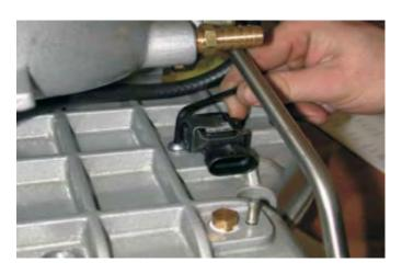
52. Remove the power brake hose and clamp from the stock intake manifold.
