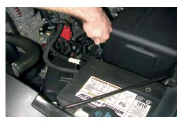
5. With a cool engine remove the radiator cap. (Be careful not to remove the cap if the engine is still hot.)
