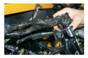
78. Route the wiring harness over the left side fuel rail and attach it to the supercharger manifold as shown, using the Adel clamp and bolt supplied.
