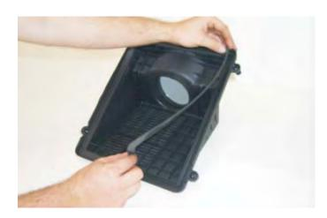
90. Install K&N air filter and reassemble the air box assembly. Reinstall the completed unit on the vehicle.
