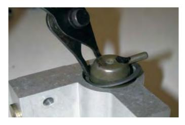
58. Apply a small amount of grease to the new supplied fuel manifold O-ring and set in the machined recessed area on the new driver side fuel rail as shown.
