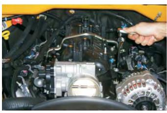
31. Carefully remove the intake manifold assembly and set aside.
