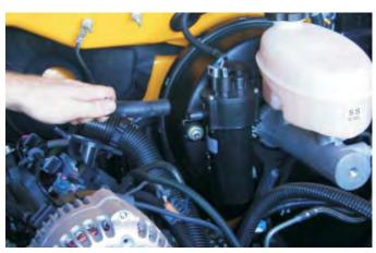
27. With the fuel line disconnect tool supplied, remove the fuel line from the fuel rail. Caution! The system may be under pressure. Avoid open flame or other sources of ignition.
