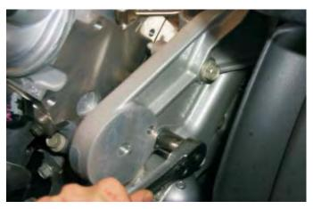
69. Install the tensioner and it's mounting bolt on the new mounting bracket. Torque the tensioner mounting bolt to 50 lb-ft.
