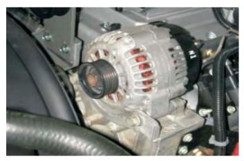
85. Reattach the battery cable to the alternator terminal.
