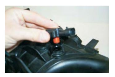
50. Put some lubricant on the MAP sensor seal and press the MAP sensor into the provided hole in the supercharger manifold as shown.
