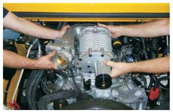
73. Remove the 10 spilt looms that support the fasteners. Start all <u>ten bolts</u> by hand.
