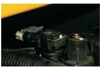
23. Disconnect the engine knock sensor connector and steel-mounting clip from the intake manifold by prying it free with a small screwdriver. Next, gently raise the black plastic retaining clip and then pull free the connector from the harness.
