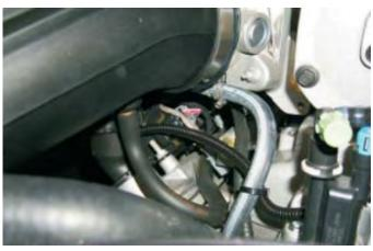
97. Locate MAF cable, pull back flex loom approximately 8 inches. Separate the tan & black wires from this harness.
