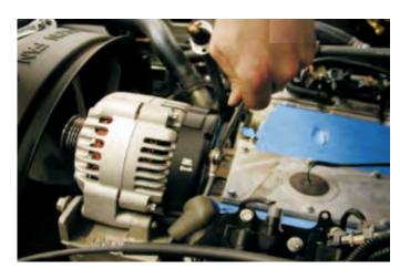
40. With a 15mm socket wrench remove the two bolts holding the alternator to the alternator bracket. Remove the alternator.
