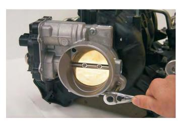
62. Install the three studs removed in the previous step into the new supercharger inlet manifold using a #5 internal Torx socket and wrench.
