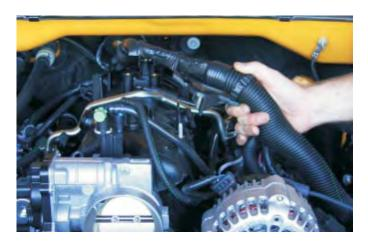
26. Remove the power brake hose from the control valve. (Some vehicles have hydraulic assist and do not have this hose.)
