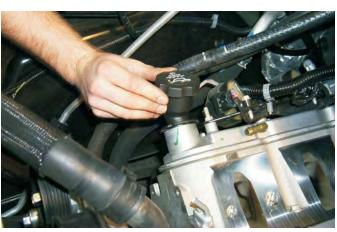
43. Take the new supplied coolant vent pipe and test fit to the front of the cylinder heads. Check for clearance between the pipe and the alternator bracket as shown.
