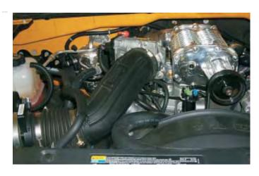
96. Attach the PCV hose from the right (passenger) side valve cover to the brass barb on the bottom of the air tube. Connect the PCV hose from step 47 to the remaining barb next to the power brake hose connection on the back of the inlet manifold. Connect the power brake hose to the control valve shown in step 26.
