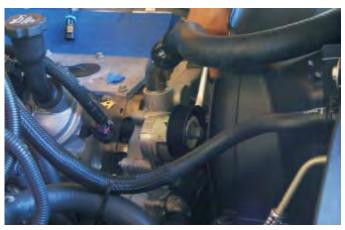
39. Using a 10mm wrench disconnect the battery positive terminal from the back of the alternator.
