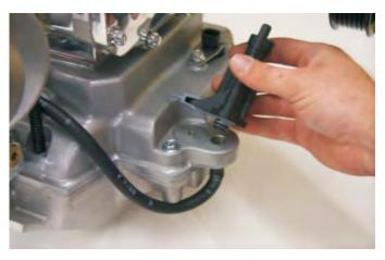
65. Mount EVAP solenoid on front of intake manifold.
