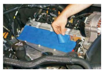
34. Using a 15mm wrench, remove the steel bracket from the rear of the driver side cylinder head. This will not be reused.
