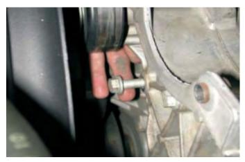
67. Here is the new tensioner support bracket and hardware. The new bracket will locate in the original tensioner location. Note: The different fasteners and their locations.
