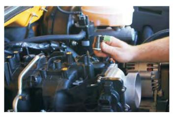
29. Remove the Positive Crankcase Vent (PCV) vacuum hose from the intake manifold on driver side.
