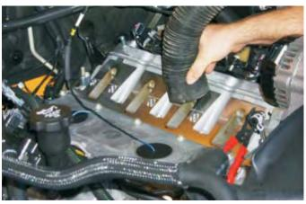
33. Cover the intake ports with tape or clean rags to keep dirt and objects from entering the engine. (Remember, be clean.)
