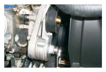
70. Install the 90mm idler and spacer on the idler support bracket. Torque the mounting bolt to 40 lb-ft.
