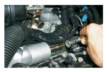
76. Using supplied gasket, mount throttle body using stock nuts and torgue them to 89in-lbs.
