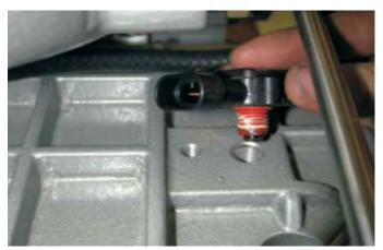
51. Using a 4mm allen wrench, install the MAP sensor retaining clip with the provided 6mm button head screw as shown.
