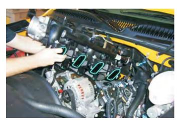
32. Using a vacuum cleaner, remove any dirt or debris from the intake port area. (Be careful not to get any dirt in the intake ports.)
