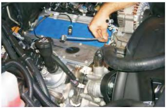
37. Using a 15mm tensioner wrench or breaker bar, remove the stock serpentine belt from the vehicle. The belt will not be reused.
