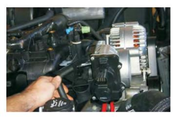
17. Using a 10mm socket wrench, remove the three bolts that fasten the cover support bracket from the top of the intake manifold.
