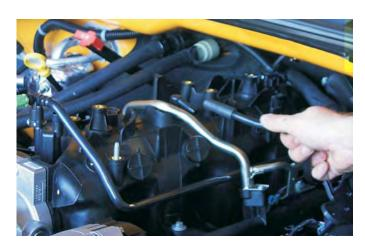
30. Using a 8mm socket wrench remove the ten intake manifold bolts.
