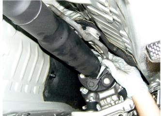
Carrier shown completely removed.
