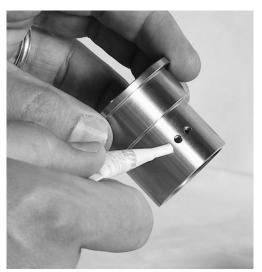
Install the unit into the carrier on top of the white bushing.
