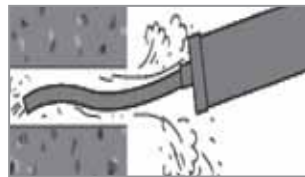
02 Blow out dust and fragments.
