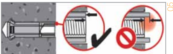
05 Make sure the anchor is flush against the surface.
