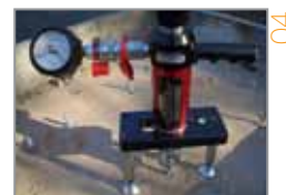
04 Conduct a pull test on each anchor using the Hydr jaws testing kit to 6kN.
