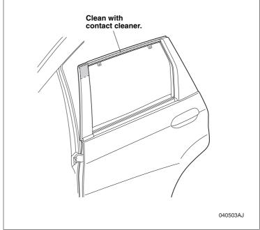
17. Remove the adhesive backing from each sealer, and attach them to the left rear door as shown.
