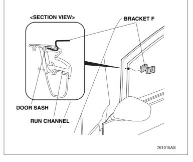
29. Install the bracket F between the door sash and the run channel in the position shown.
