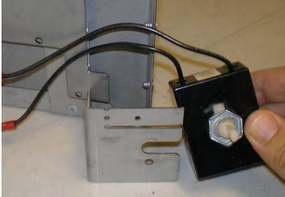
1 Remove Fan Control Switch From Current Position.
