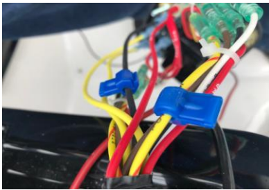
Shows T-Tap connectors in place
