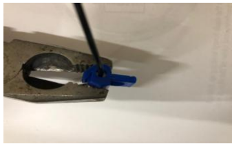
Shows T-Tap connectors in place
