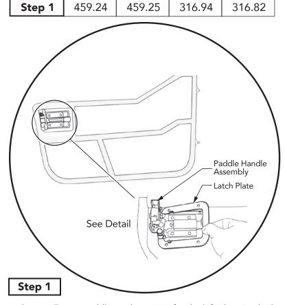
In this installation, Paddle Latch #459.24 fits the left (driver) side door, and Paddle Latch #459.25 fits the right (passenger) side door.
