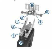
2 Attach the transducer mount bracket to the transom mount bracket (5) using the bolts (6), flat washers (7), and lock nuts (8).
