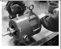
Fig. 11-11: Tap Out Shaft Assembly
