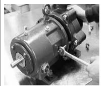
Fig. 11-3: Bolts to Connect Bearing Frame
