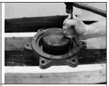
Figure 8-8: Remove Containment Shell
