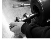
Fig. 11-12: Remove Shaft Assembly
