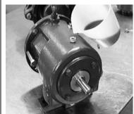
Fig. 11-22: Fill Bearing
