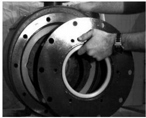
Figure 9-8 Placing back plate on casing
