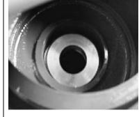
Figure 11-16: Install Labyrinth Seal into Cavity
