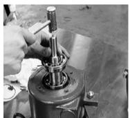
Figure 11-19, Insert Shaft Assembly into Bearing Frame
