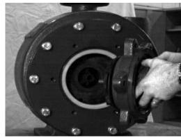
Figure 9-10 Assembling impeller/rear casing
