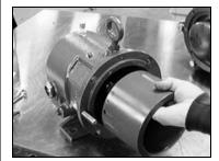
Fig. 11-7: Slide Outer Drive off Shaft or OMR from Adapter Hub
