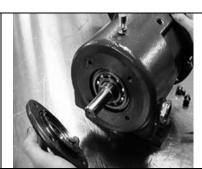
Fig. 11-10: Remove Bearing Cap
