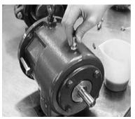
Fig. 11-21: Remove Breathing Tube
