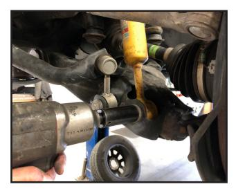
10. Remove the 2 bolts that attach the lower ball joint to the bottom of the steering knuckle.
