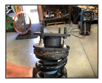
16. Locate the new 3/8" flange nuts, Reinstall the struts back into the vehicle and loosely start the new 3/8" flange nuts. Do not tighten at this time.
