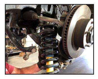
17. Raise up the lower control arm so that the lower strut bolt can be reinstalled, Do not tighten at this time.
