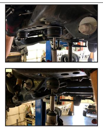
4. Carefully lower the front differential down approximately 3/4" to install the new spacer sleeves.
