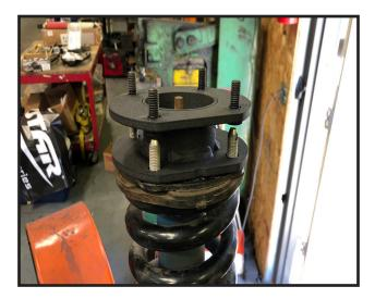
15. Secure the new spacers using the OE nuts
