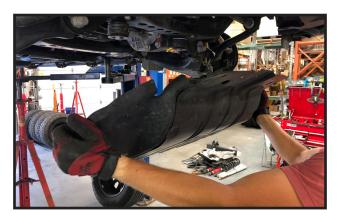
3. Locate the 2 front mounting brackets for the differential. Using a suitable jack to support the front differential, remove the OE mounting hardware that goes through the crossmember. **The OE bolts and nuts may be discarded**, **but keep the OE oversized washers**.
