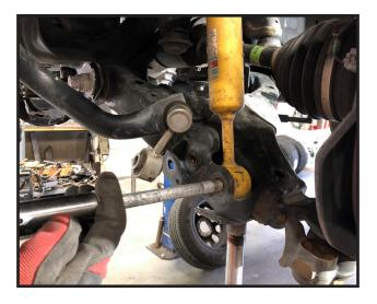
12. Remove the 4 upper strut mounting nuts. Special note: make sure the lower control arm is propertly supported so the suspension doesn't drop out when these nuts are removed.
