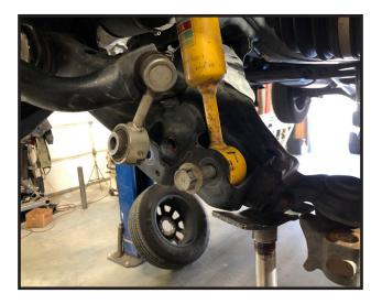
18. Carefully raise the lower control arm up so that the lower ball joint bolts can be re-installed into the steering knuckle. Torque to 160 ft lbs. Special note: While performing this step, it requires the front suspension to be compressed greatly, so its recommended that a stabilizer jack be placed under the rear bumper or trailer hitch of the vehicle to prevent it from pivoting.
