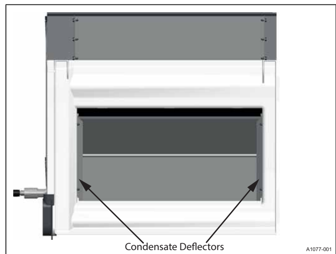
FIGURE 12: CM60C Horizontal Right Coil Condensate Final Assembly
