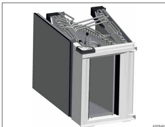
FIGURE 9: Recommended Position of Coil to Install Downflow/Horizontal Right Condensate Components
