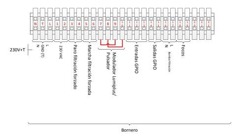
**Figure 2: Fluidra Connect terminal block**
