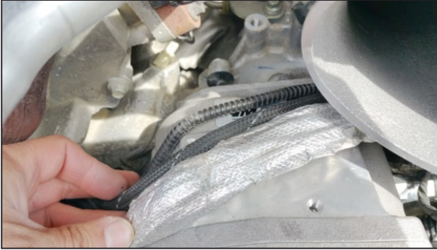
Figure 12 — Installing the cable tray (V300011 compressor shown)
