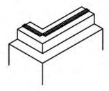
INCORRECT - Do not overlap the rubber sealant material at a corner. Rubber sealant should be continuous around corners.
