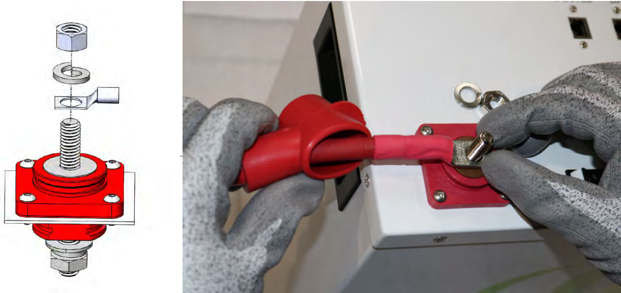
Figure 7.0 – Cable Lug Wiring onto AmpliPHI Threaded Stud
