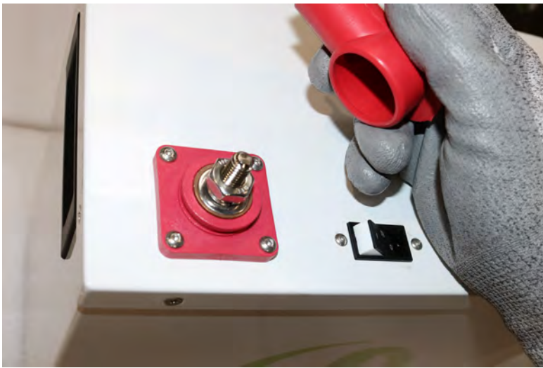
Figure 3.0 – AmpliPHI Threaded Stud
