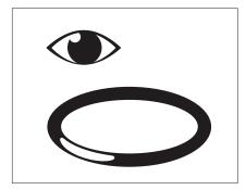
► Visually inspect replacement sealing element. Ensure there are no defects, scratches, or burrs, is free of debris, and is coated with lubricant.
