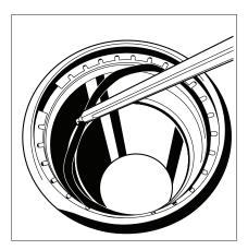
Use o-ring pick to push the sealing element into the fitting below the grip ring.
