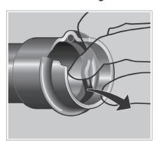
Remove the sealing element from the bead using a blunt object such as a finger or an O-ring pick.
