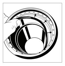
Carefully pull the sealing element up into the channel below the separator ring. Ensure proper, concentric seating of grip ring, separator ring and sealing element before installation.
