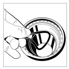
Pinch the sealing element and place it fully inside the fitting, below the separator and grip rings.
