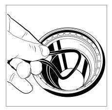
Carefully reach past the grip ring, pinch and remove the sealing element from the fitting.
