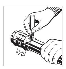
While turning slightly, slide press fitting onto the tube to the marked insertion depth.
