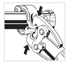
■ Hold the trigger until the Actuator has engaged the XL-C ring.
