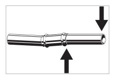
The pressing process can cause deflection (angular misalignment) to occur. When pressing Viega ProPress fittings in a system, the deformation of the fitting is constant. This allows for a consistent leak-free joint every time and is a result of the pressing technique.
