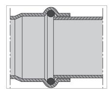
All Viega fittings are designed with cylindrical guides to keep the tube straight and protect the sealing element during assembly.
