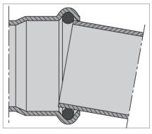
Fittings that do not have cylindrical guides risk making an unsecured connection. Without the guides, installers may damage the sealing element.
