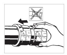
While turning slightly, slide fitting onto the tube to marked insertion depth.
