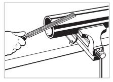
■ Use a wire brush, Scotchbrite pad, sand cloth, or sandpaper to remove loose dirt and rust particles from the pressing area.
