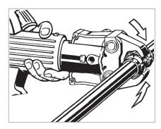
■ Hold trigger on press tool until press jaws have fully engaged the fitting. Jaws will automatically release after a full press is made.
