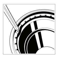
Insert o-ring pick between sealing element and separator ring.
