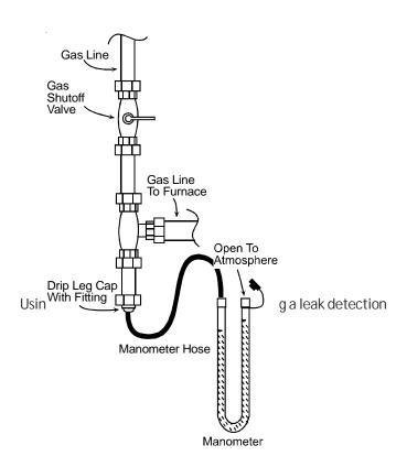
Measuring Inlet Gas Pressure (Alt. Method)
