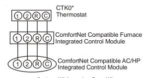
System Wiring using Four-Wires
