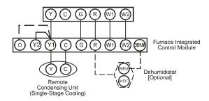
Thermostat - Two-Stage Heating with Single-Stage Cooling
