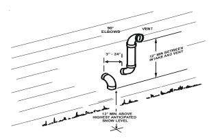
Alternate Horizontal Vent Termination (Dual Pipe)
