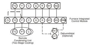
Thermostat - Two-Stage Heating with Two-Stage Cooling
