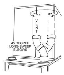
Increased Clearance Configuration Figure 9A
