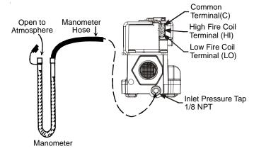
Honeywell Model VR9205 Connected to Manometer
