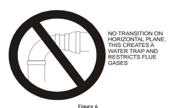
Some models require the use of 3" pipe. Do not transition from a 2" to 3" pipe in a horizontal section of pipe as this may create a water trap.
