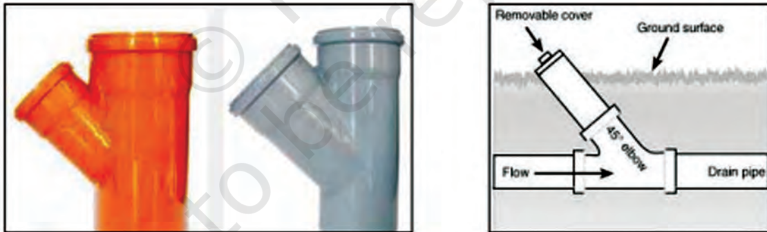
Fig. 4.4: Y-T joint
