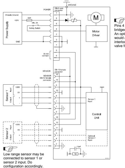
Pins 4 and 8 must be bridged for operation. An optional switch would allow for motor interlock to prevent valve from moving.
