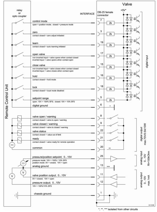
Do not connect other pins than indicated in the schematics above! Use only screws with 4-40UNC thread for fastening the DB-25 connector!
