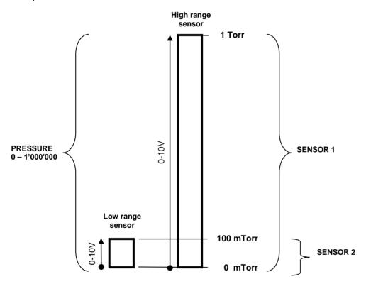
Above picture shows a 2 sensor system. In this configuration sensor 2 covers low range (100 mTorr) and sensor 1 covers high range (1 Torr).
