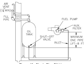
Figure 18: Single Pipe Oil Line
