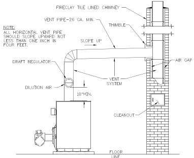
Figure 16: Recommended Smokepipe Arrangement and Chimney Requirements
