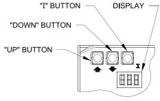
Figure 30: Boiler Control Key Function & Orientation
