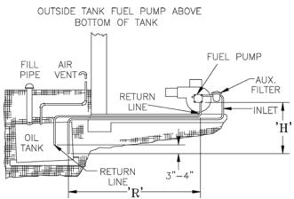
Figure 19: Two Pipe Oil Lines
