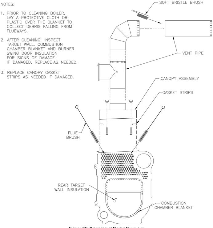
Figure 31: Cleaning of Boiler Flueways
