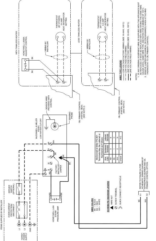
Figure 22: Schematic Wiring Diagram, Steam Boilers With or Without Tankless Heater, McDonnell & Miller PS-801 Probe LWCO, Beckett AFG Burner
