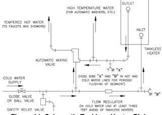
Figure 14: Schematic Tankless Heater Piping
