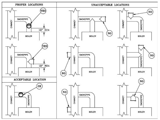
Figure 17: Proper and Improper Locations of Draft Regulator
