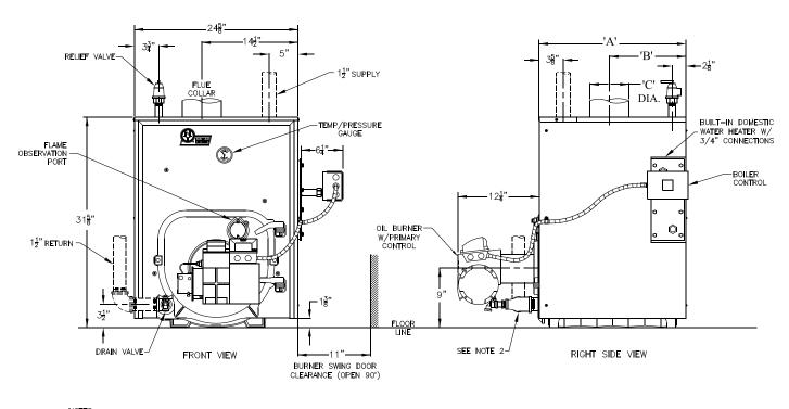
NOTES: 1. CIRCULATOR SUPPLIED LOOSE – MAY BE INSTALLED ON SUPPLY OR RETURN. 2. RETURN FITTINGS AND DRAIN VALVE SHIPPED LOOSE. 3. PIPING SHOWN HIDDEN NOT FURNISHED WITH BOILER.
