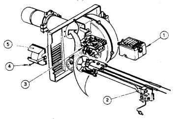
Figure 5: Installation/Removal of Riello Drawer Assembly
