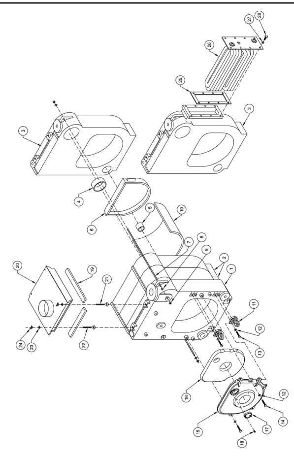
Bare Boiler Assembly (Exploded View)
