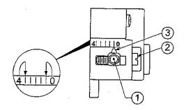
Figure 8: Riello Turbulator Setting
