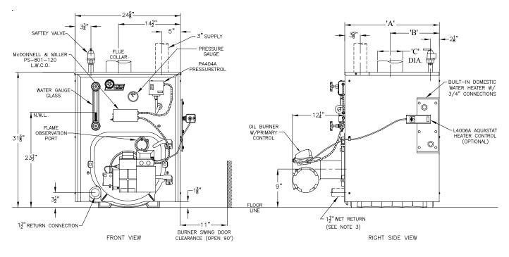
NOTES: 1. TANKLESS COIL OPENING NOT PRESENT ON LESS-COIL BOILERS. 2. PIPING SHOWN HIDDEN NOT FURNISHED WITH BOILER. 3. DRAIN VALVE SHIPPED LOOSE. (NOT SHOWN)
