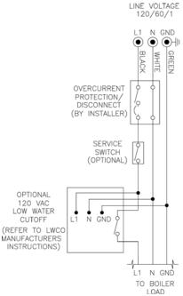
Figure A2: Wiring of Typical LWCO
