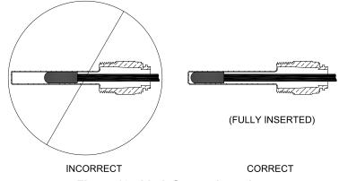
Figure 10: Limit Sensor Insertion
