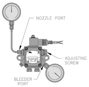
Figure 25: Adjusting Fuel Pump Pressure
