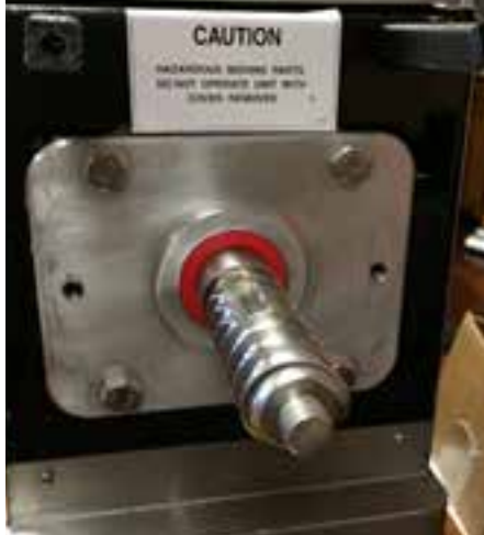
Wipe the auger, rotary seal and housing mounting plate thoroughly using a dry cloth
