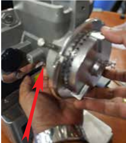
Press/Hold Auger lock pin. Rotate Grinding Wheel counterclockwise.
