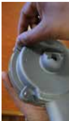
Unscrew 3 captive screws, and separate the retaining ring from cover for cleaning. When reinstalling these pieces, make sure the raised weld nuts do not rest against the cover when hand tightening the retaining ring and 3 thumb screws. Failure to do so, may result in leaking.
