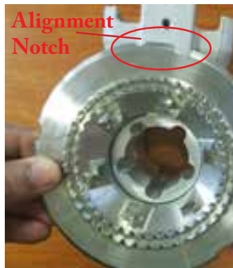
Unscrew the two thumb screws which hold the grinding plate on the auger housing and remove for cleaning. Take notice of the alignment notch which needs to be located in the range as shown by the red circle during the reinstallation process.
