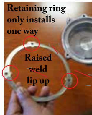
Unscrew 3 captive screws, and separate the retaining ring from cover for cleaning. When reinstalling these pieces, make sure the raised weld nuts do not rest against the cover when hand tightening the retaining ring and 3 thumb screws. Failure to do so, may result in leaking.
