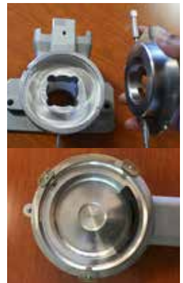
Unscrew the two thumb screws which hold the grinding plate on the auger housing and remove for cleaning. Take notice of the alignment notch which needs to be located in the range as shown by the red circle during the reinstallation process.
