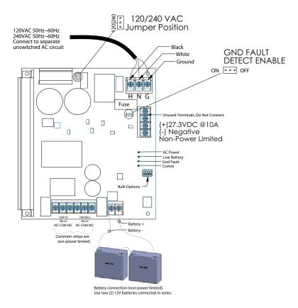
Primary AC 120VAC 50Hz~60Hz, 5.1AMP Min Low AC Detect 97VAC 240VAC 50~60Hz 2.5AMP Min Low AC Detect 190VAC
