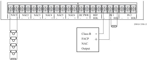
Class A Trigger and Class A Notification Circuit
