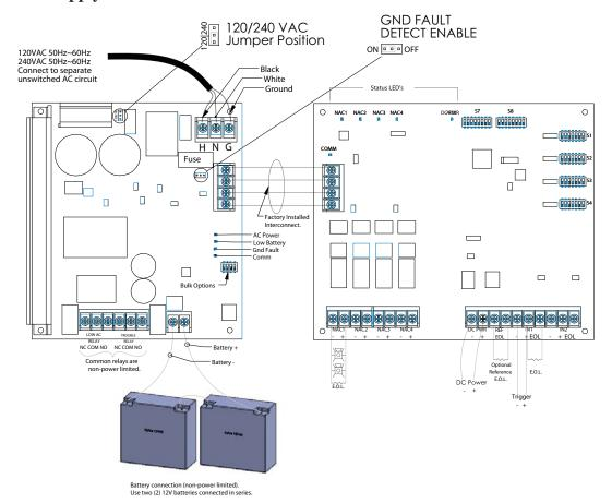
Primary AC 120VAC 50Hz~60Hz, 5.1AMP Min Low AC Detect 97VAC 240VAC 50~60Hz 2.5AMP Min Low AC Detect 190VAC
