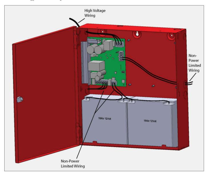
**Note:** The output of the bulk power supply is not power limited. All field wiring must be a minimum of 18 AWG and installed in conduit. All wiring connections must be made within 20 feet (6.1 meters) of the bulk supply.
