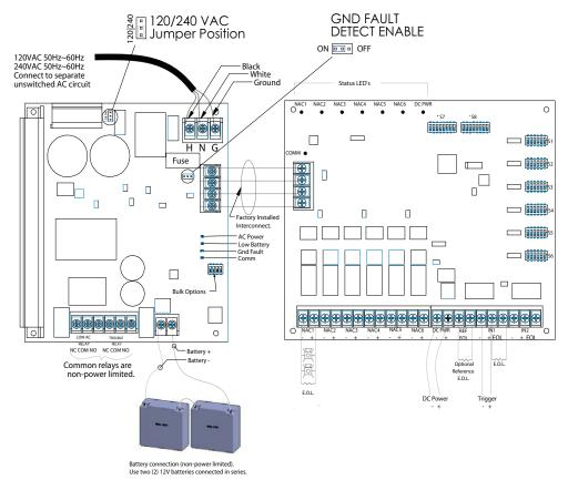
Primary AC 120VAC 50Hz~60Hz, 5.1AMP Min Low AC Detect 97VAC 240VAC 50~60Hz 2.5AMP Min Low AC Detect 190VAC
