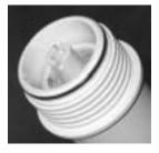
You must change the flow restrictor each time you change the Membrane filter. Replace the existing flow restrictor with the new one by removing the White compression nuts. Make sure the arrow is pointing toward the check valves and hot water line fitting.
