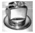
Small brass tee can be turned 1/2 turn counterclockwise, to adjust the tension on the black lever. This adjustment may be necessary to stop slow drips from tip of faucet. You may need to repeat the process until the faucet does not drip. Brass tee must always end up facing across body of faucet in order to slide black lever on.
