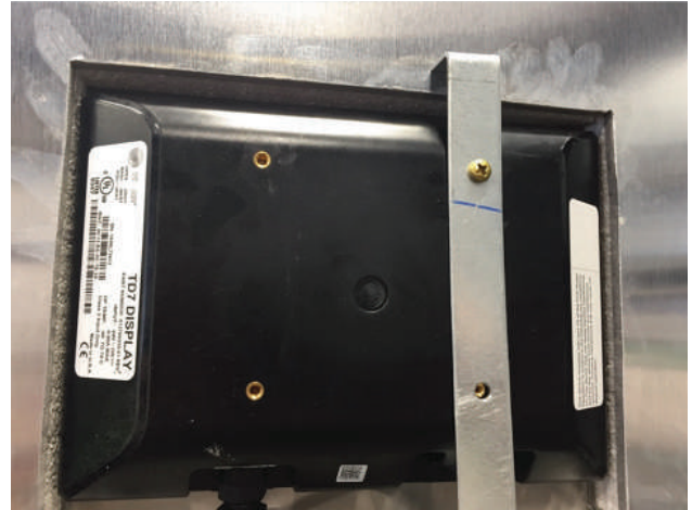
Figure 33. TD-7 Installation on back with brackets
